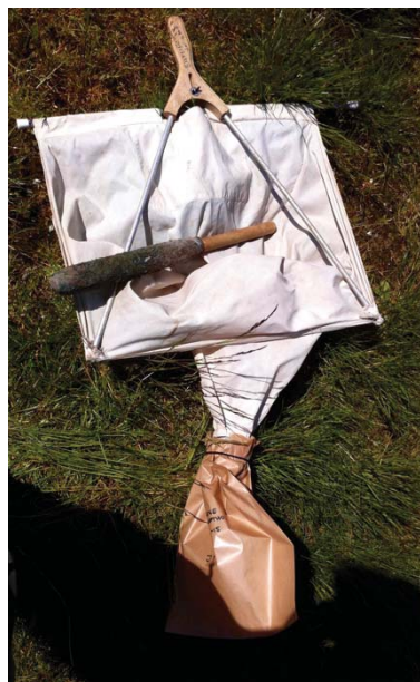
Figure 5: A Styrofoam covered stick was used to tap one branch three times each. This treatment dislodged insects into the funnel that had a paper bag connected at the end.
