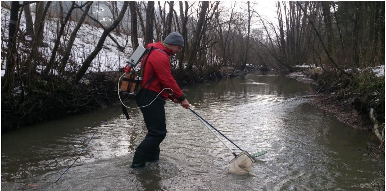
Figure 3: Electrofishing conducted at station 3 in winter at lower water discharges. A handhold net is held close to the anode to capture any stunned fish.
