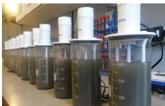
Figure 11: Setup of jar-test apparatuses during the experimental work of this thesis.
