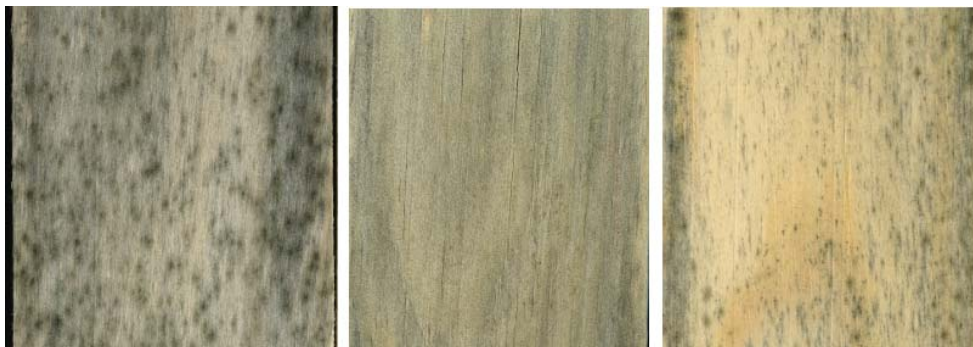
Figure 1. Surface mould growth on three different specimens of pine sapwood.
