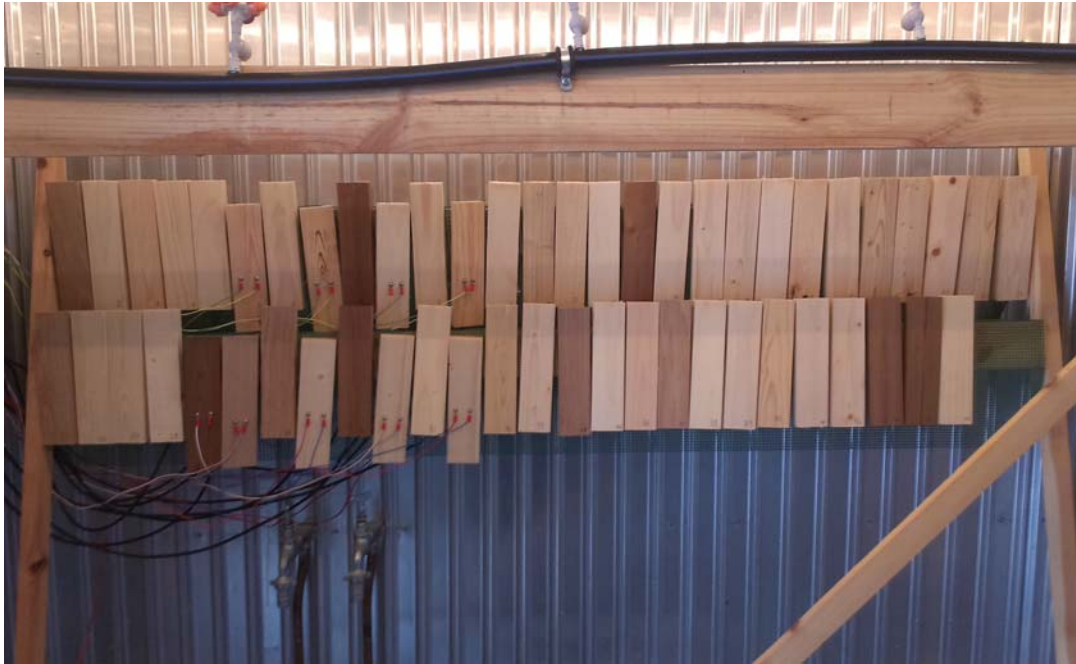
Figure 5. Test rig with specimens. As this experiment was a part of a larger project, there were more specimens on the rig than what was studied in this thesis.
