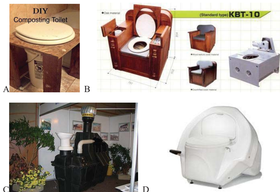
Figure 5. Examples of different composting toilets. A – simple homemade composting toilet (Kathryn @ Farming My Backyard, 2014), B – Bio-Lux toilet (Japan)(Seiwa Denko, 2003), C - Enviro Loo - Waterless composting toilet system (South Africa)(SuSanA Secretariat, 2005), D – Naturum, model produced by Bioland (Finland)(Biolan, 2014).
