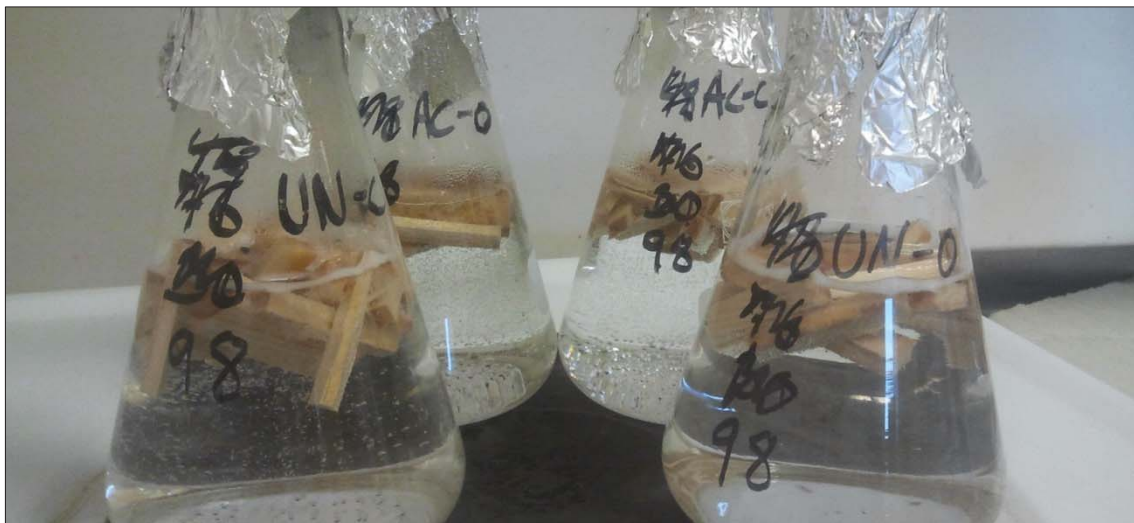
FIGURE 23: BOILING OF WOOD CHIPS FOR EXTRACTION OF EXTRACTIVES, UNTREATED IN FRONT AND ACETYLATED BACK. FOAM IS CREATED IN THE FLASKS WITH UNTREATED WOOD.
