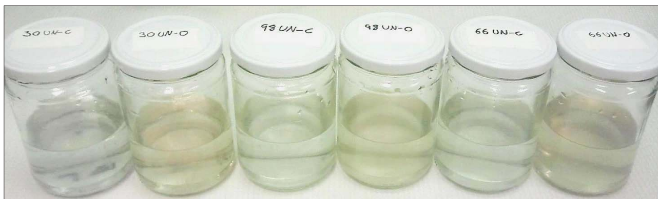
FIGURE 24: COLOUR OF WATER FROM THREE UNTREATED PLANKS AFTER EXTRACTION, UN = UNTREATED, C = CORE AND O = OUTER PART.
