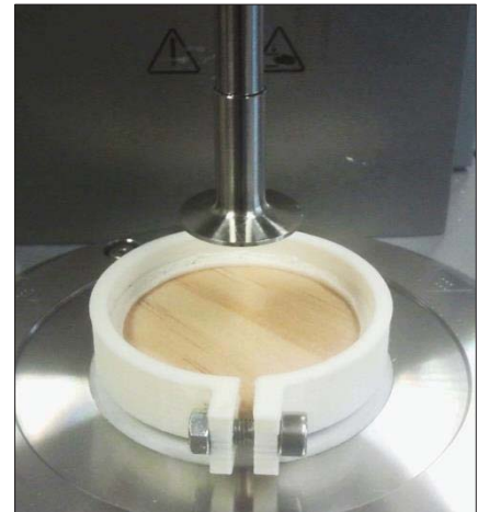
FIGURE 6: 3D PRINTED HOLDER TO FIXATE THE WOOD DISCS ON THE RHEOMETER
