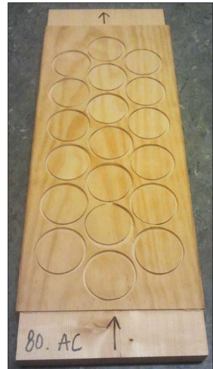
FIGURE 4: FRESHLY PLANED AND CUT ACETYLATED DISCS PREPARED FOR RHEOLOGY TESTING
