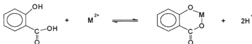
Figure 3.7: Mechanism between humic acid and metals (Dupay and Douay, 2001).
