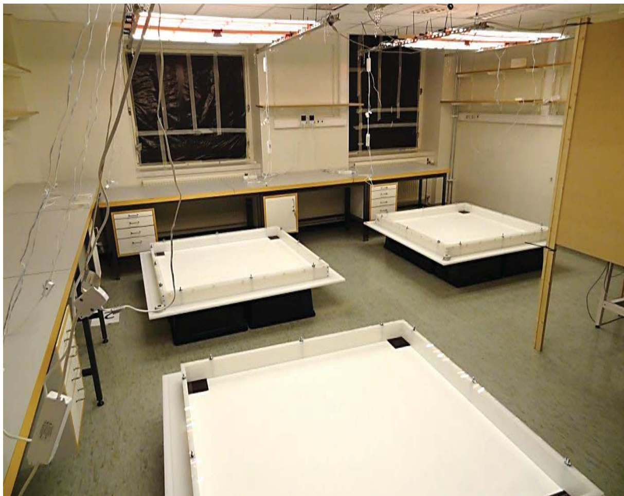
Figure 4. Arena studies with three arenas in the same room. Dark squares in the corner are hiding places for the bed bugs. Light and camera mounted straight above all three arenas.
