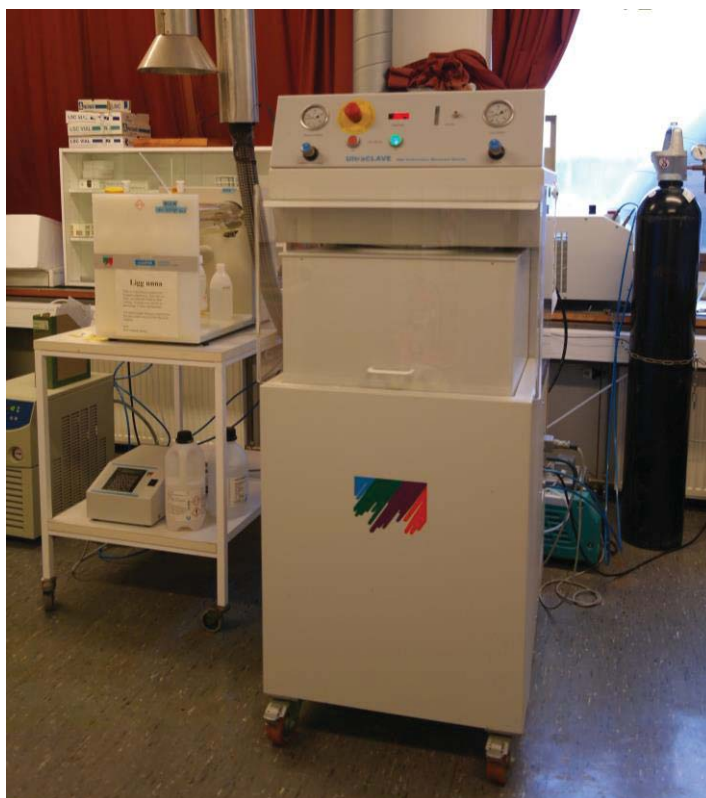
Figure 10: Ultra Clave High Performance Microwave Reactor by Milestone Incorporated, Shelton, USA
