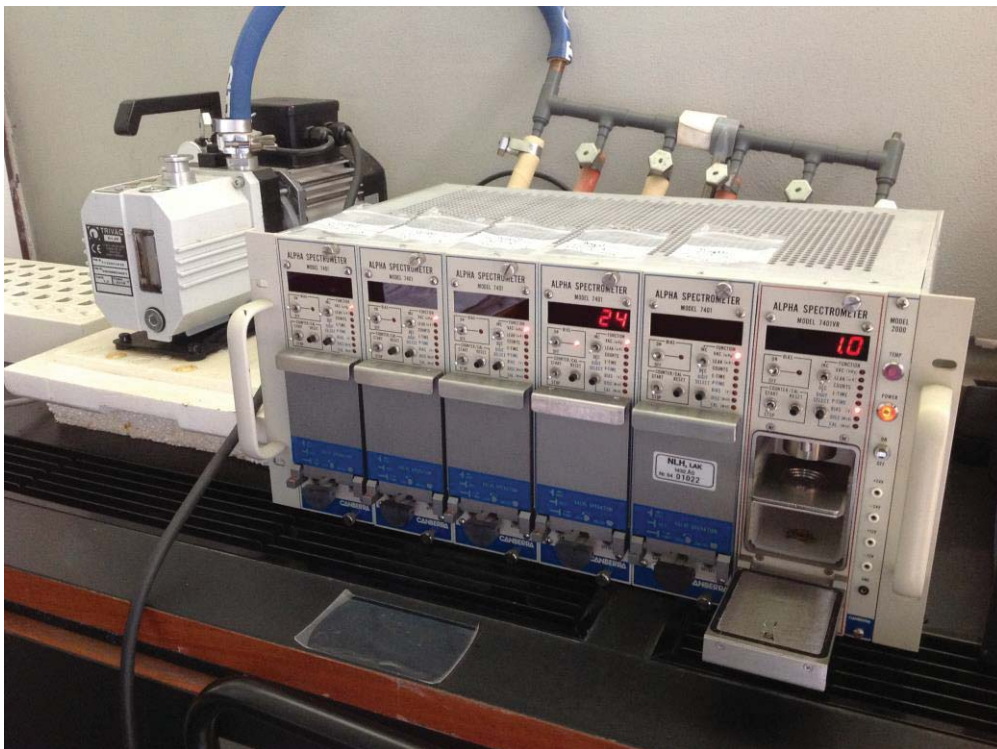
Figure 13: VR 740 Alpha spectrometer by Canberra, Sidney, Australia
