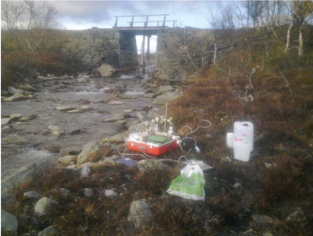
Figure 7: Sampling and fractionation in situ (Site 1) in River Orva located near the outlet of River Orvsjøen 1 km upstream of the Kongens area.
