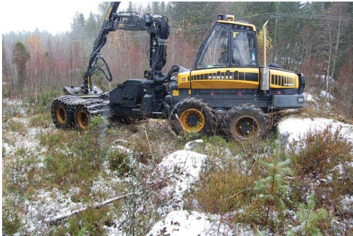
Figur 12. Ponsse Dual kombimaskin
