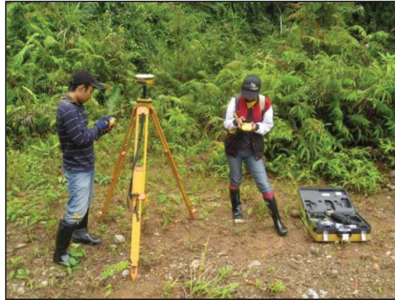
Figure 9. Work with Topcon Hiper II GNSS-receiver in the road close to one of the sample plots
