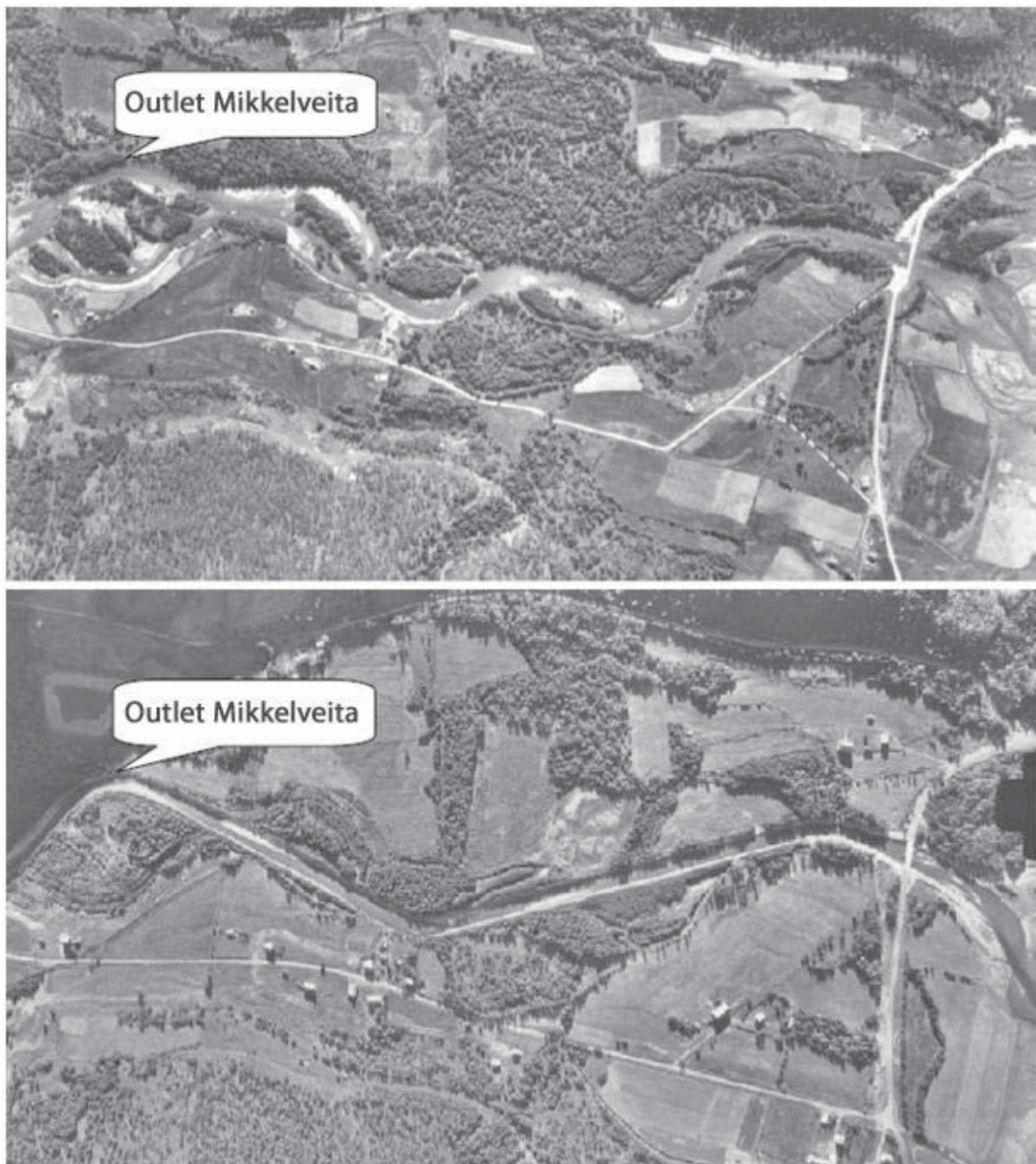
Figure 2. Orthophoto over the same lower section of the Bognelva river taken in 1946 before channelization (top) compared to after channelization over many years taken in 1972 (bottom) (Norges Flyfoto arkiv).
