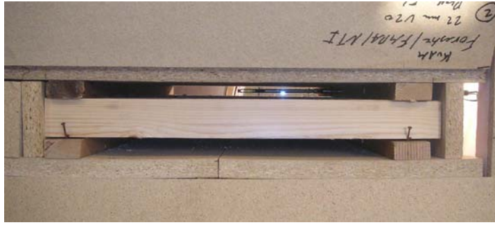
Figure 11. The samples shown from the in blowing side with air velocity meter in center of the upper sticker layer.
