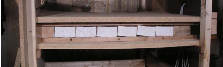
Figure 8. Six samples in each run were placed between two fiberboards and stickers.
