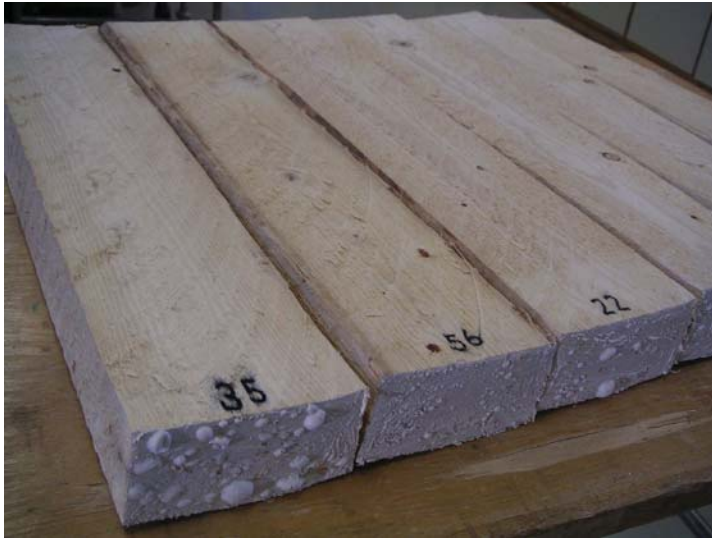
Figure 7. The six 50 by 100 mm boards were cut into 500 mm lengths and sealed at the ends with silicone. Numbers refers to board number and position in board.
