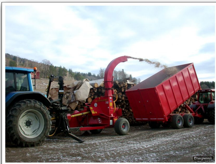
Figur 3. Junkkari HJ 500 Contractor flishogger (Kilde: Energiveven).
