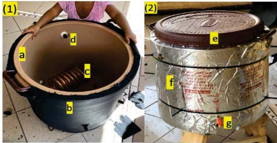
**Figure 3.5:** Some details of thermal storage vessel showing: (a) the thermos vessel, (b) armafex insulation, (c) heat exchanger, (d) spout for transducer insertion, (e) non modified lid, (f) thermal resistant foil cover and (g) manual valve
