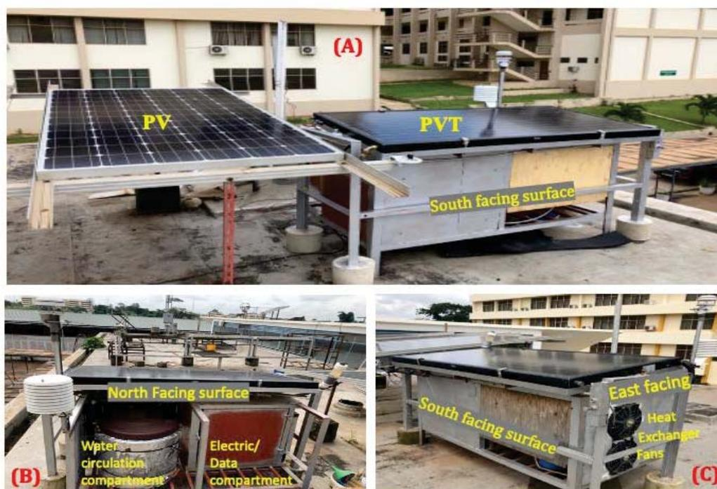
**Figure 3.10:** Installation of setup on the roof top of Solar Energy Applications Laboratory at Department of Mechanical Engineering, KNUST Ghana, showing; (A) PV and PVT modules; (B) North facing surface with water circulation and Electric/Data compartments; (C) East facing surface with radiator cooling fans
