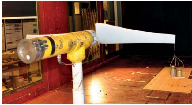
Figure 2.14: Calibration process of torque transducer.
